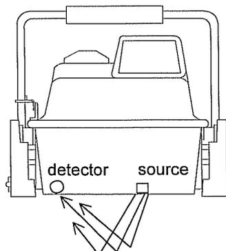
The Geiger Mueller detector inside the meter measures the amount of gamma radiation reflected, or "scattered back", from the material in terms of counts per minute (CPM).
